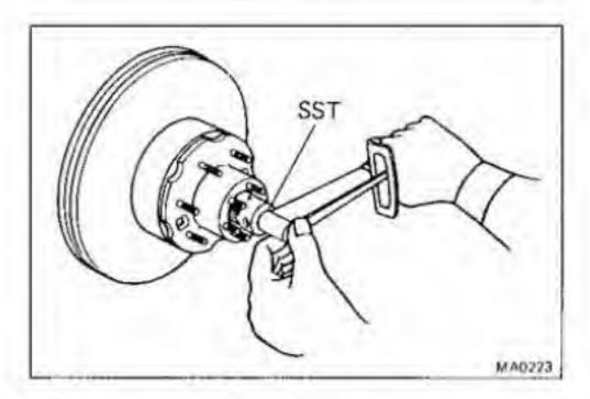
(e) Using SST, tighten the lock nut.
